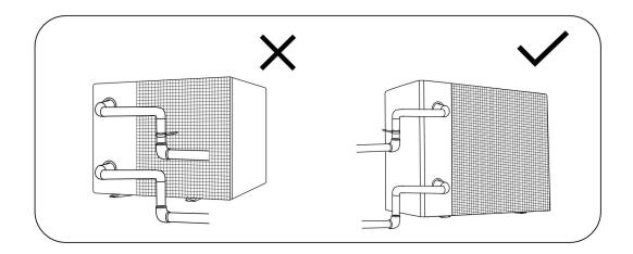
DO NOT install water pipes in a way that they pass behind the heat pump's evaporator. In case this cannot be avoided, cover the pipes with thermal insulation foam.
