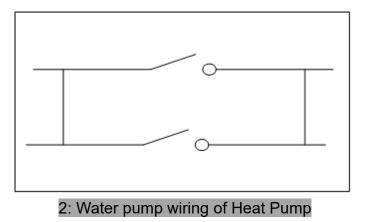
Note: The installer should connect 1 parallel with 2 (as above picture). To start the water pump, condition 1 or 2 is connected. To stop the water pump, both 1 and 2 should be disconnected.
