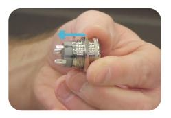
Fix the button using the locking nut to secure it to the back of the cabinet panel.
