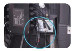
Step 7: Connect power supply to amplifier. Connect the white two-pin connectors.
