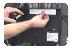
Step 5: Using four small screws attach Amplifier to the black box.
