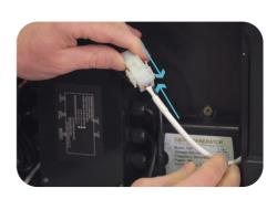
Step 8: Connect power supply to the SpaNet™ controller
