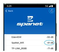
NOTE: During the setup process you can use the refresh arrow in the top right corner to perform another WiFi scan and update the dB signal readings (refer picture above). This can be helpful if you are trying to determine the best position for mounting your SmartLink™ module or router.
