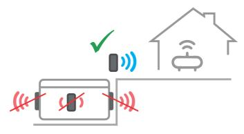
Note: Longer data cable may be required. Do not extend existing data cable, replace if longer length required, maximum cable length = 10m.
