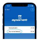
NOTE: If no WiFi network found, relocate module to a better position and use the refresh button to conduct a new WiFi scan to see if signal has improved. Signal strengths closer to 0 are stronger. If problems are experienced go Back and re-start process.
