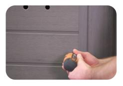
Push the SmartLink™ connector cable through one of the holes.
