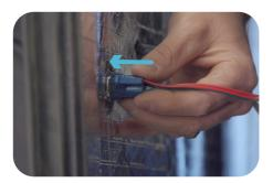
Step 15: Connect the SmartLink™ antenna into the SpaNet™ controller.
