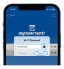
NOTE: Take care when entering password, the SmartLink™ module or app cannot check or verify the password. It relies on correct entry. If the password is incorrect, you must delete the spa instance and start the setup process again.
