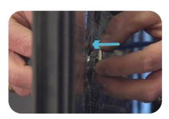
Complete the final connection by plugging the button into the connector on the back.
