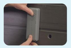
**NOTE:** The module MUST be positioned in a vertical orientation, with the WiFi symbol at the top to maintain waterproofing and for best signal strength.
