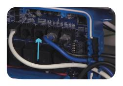
Expansion port 1 is the third port from the right. Also, labeled underneath the port as Exp 1.
