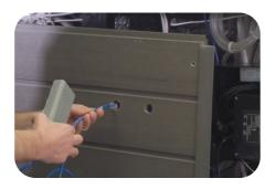
Use the adhesive backing from the module to secure it into the spa cabinet.
